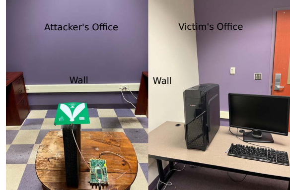
Fig. 6. Setup for the wall-penetrating model extraction attack.
